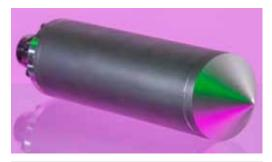
Diameter 76mm Length 300mm Temp Range -50°C to + 125°C Frequency Response 4Hz to 400Hz Voltage Sensitivity 10V/g
