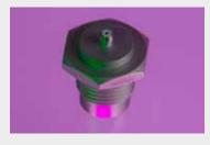
M/02/F, M/02/T Sensitivity 5nC/bar nom. Weight 46gm (F) 70gm (T) Size (mm) 23 (F) 33.5 (T) Min-Max. Temp -50°C • 250°C Max Wkg. Pressure 200 bar Deviation -5% @ -50°C +15% @ +250°C
