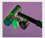
IH-10 Sensitivity 0.5mV/N Measuring Range 1000N Hammer Mass 750gm Head Diameter 32mm Hammer Length 340mm Output Connector BNC Tips Supplied Hard tip, Medium tip, Soft tip
