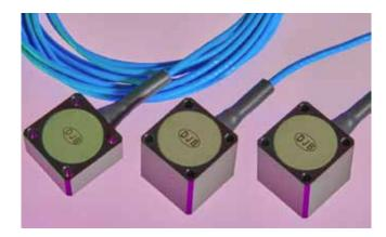
The AM range of accelerometers are MEMS (micro electro mechanical system) DC response devices for testing low frequency vibration measurement from DC (0Hz) and above. They are a variable capacitance design and are available with a 2m integral cable fitted with a 7 pin connector to suit the DJB DCM-03 MEMS signal conditioning unit or alternatively as bare wires.
