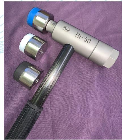
The IH-50 impact hammer belongs to a range of general purpose hammers used for structural health testing, resonance determination and modal analysis, the IH-50 itself being suitable for more heavyweight testing. Included within the hammer is a piezoelectric IEPE force sensor in which directly outputs a voltage signal.
