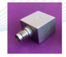
A lightweight general purpose PE charge output tri-axial vibration transducer comprising of three charge output Konic Shear® piezoelectric sensing elements mounted orthogonally within a titanium block with fully welded construction. The AT/04 is one of only 3 PE charge output single connector accelerometers in the world, all produced by DJB Instruments. This is possible due to the unique low noise four core cable supplied by DJB to reduce triboelectric noise.
