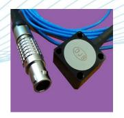
The AMT range of accelerometers are Triaxial MEMS (micro electro mechanical system) DC response voltage output devices for testing at low frequency vibration measurement from DC (0Hz) and above. They are Triaxial (measuring in 3 directions simultaneously) variable capacitance design and are available with a 2m integral cable fitted with a 7pin connector to suit the DJB DCM-03 MEMS signal conditioning unit or alternatively as bare wires.
