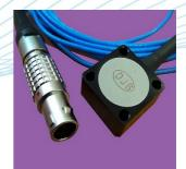
The AMB range of accelerometers are Biaxial MEMS (micro electro mechanical system) DC response voltage output devices for testing at low frequency vibration measurement from DC (0Hz) and above. They are Biaxial (measuring in 2 directions simultaneously) variable capacitance design and are available with a 2m integral cable fitted with a 7pin connector to suit the DJB DCM-03 MEMS signal conditioning unit or alternatively as bare wires.
