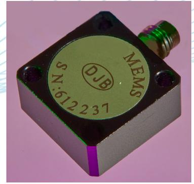
The AMB range of accelerometers are Biaxial MEMS (micro electro mechanical system) DC response voltage output devices for testing at low frequency vibration measurement from DC (0Hz) and above. They are Biaxial (measuring in 2 directions simultaneously) variable capacitance design. The AMB/20.100C has a 4 pin ¼-28UNF side entry connector.
