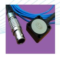
The AM range of accelerometers are MEMS (micro electro mechanical system) DC response voltage output devices for testing at low frequency vibration measurement from DC (0Hz) and above. They are single axis variable capacitance design and are available with a 2m integral cable fitted with a 7pin connector to suit the DJB DCM-03 MEMS signal conditioning unit or alternatively as bare wires.
