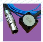
The AM range of accelerometers are MEMS (micro electro mechanical system) DC response voltage output devices for testing at low frequency vibration measurement from DC (0Hz) and above. They are single axis variable capacitance design and are available with a 2m integral cable fitted with a 7pin connector to suit the DJB DCM-03 MEMS signal conditioning unit or alternatively as bare wires.
