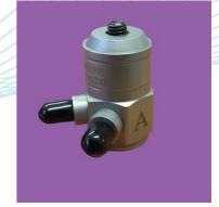
The AF/50/5 Impedance head integrates an IEPE accelerometer and force sensor into one device to measure dynamic acceleration and force simultaneously.
