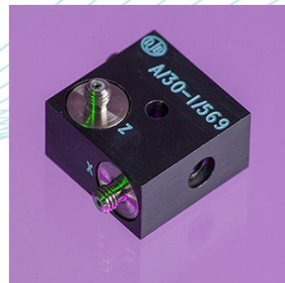
General purpose triaxial vibration transducer comprising three welded Konic shear® sensing elements bonded orthogonally into hard anodized aluminum housing. The inserts are electrically insulated individually and from the housing, thus eliminating ground loop interference.
