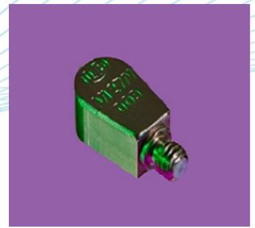
Sub-miniature teardrop charge output accelerometer. Manufactured in Titanium and features an all welded construction for a robust build. Using the DJB unique Konic shear® sensing element the low mass of the A/27/E renders it transparent in the vast majority of light weight structure vibration measurement applications.
