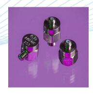
The A/24/E-1 is a miniature adhesive mount PE charge output accelerometer, offering a small size and low mass of just 2grams. Using DJB's unique Konic shear® ceramic design offering superior cross axis control and performance. The integral ceramic base provides complete electrical isolation from the surface of the test object.
