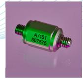
Developed for demanding applications requiring the measurement of high amplitude, short duration transient events such as pyrotechnic shock or high energy impacts, the A/16X range of stainless steel IEPE accelerometers have a range from 10,000g up to 50,000g.
