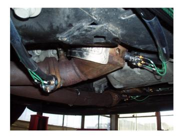
Supplied with cooling water via a windscreen washer pump the accelerometer cables and cooling pipes were protected by trunking to avoid damage under the vehicles during road tests, these were routed back to the instrumentation and pump/water supply within the vehicle.
