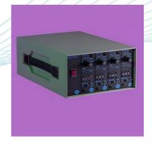
Housings for up to ten single width modules including a power supply, input/output signal connectors, module interconnections, for any practicable module combination.
