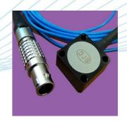
The AM range of accelerometers are MEMS (micro electro mechanical system) DC response voltage output devices for testing at low frequency vibration measurement from DC (0Hz) and above. They are single axis variable capacitance design and are available with a 3m integral cable fitted with a 7pin connector to suit the DJB DCM-03 MEMS signal conditioning unit or alternatively as bare wires.
